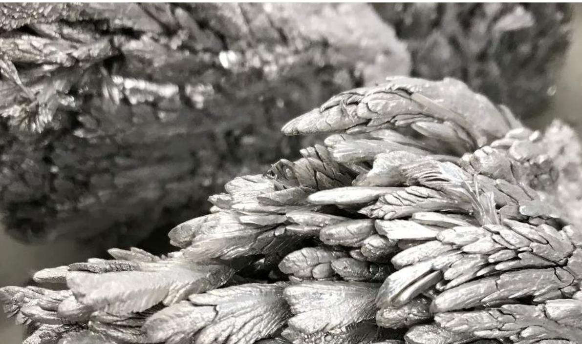
Magnesium has manifold applications in our modern society. Besides the use as high-tech material in the automotive industry, Magnesium is of great importance for the production of high-quality steel. Magnesium has a high affinity to Sulfur. This is why Magnesium has been used as an efficient desulfurizing reagent for more than 50 years. ALMAMET has been amongst the pioneers produce and promote Magnesium for the hot metal desulfurization worldwide.
